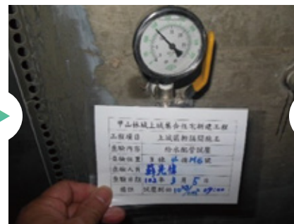
Pressure testing of each household's water supply system
